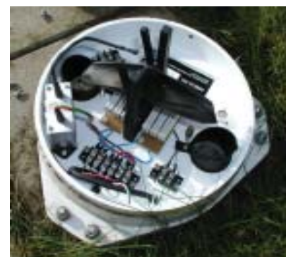
Internal view of the SBS500H high-quality rain gauge with heater
