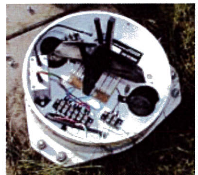
Internal view of the SBS500H high-quality rain gauge with heater
