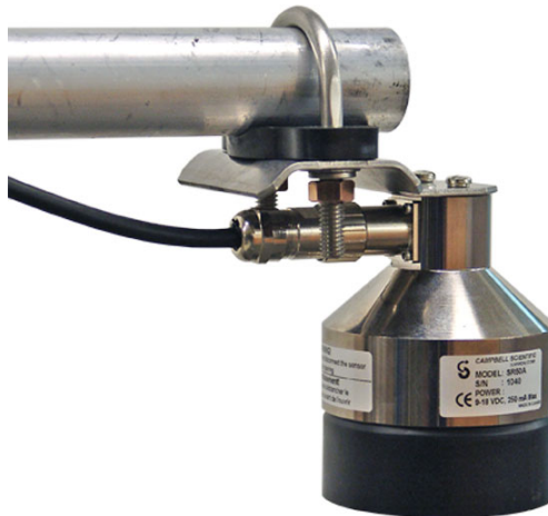
FIGURE 4-12. SR50A Mounted to a Crossarm via the 19517 Mounting Kit
