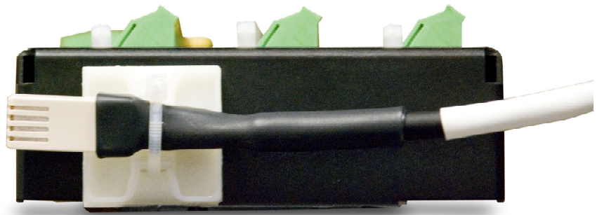
FIGURE 4-18. CS210 Installed on a CR1000
