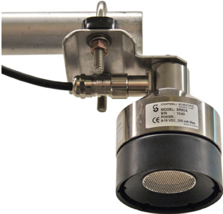
FIGURE 4-13. The SR50A Mounted to the Crossarm Shown from Another Angle
