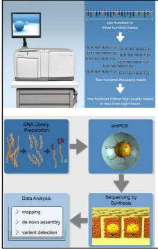
INTRO- Genome Sequencer FLX System from Roche Applied Science and 454 Life Sciences. With a read length of **200 to 300 bases** depending on organism and application parallel sequencing of over **400 000 reads**, a single run typically yields over **100 M high quality bases in less than eight hours**.
