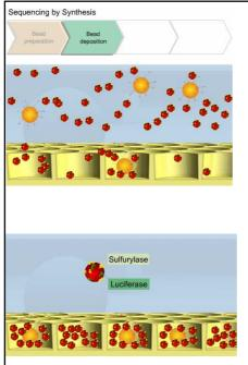
The DNA beads are layered onto a PicoTiterPlate device, depositing the beads into the wells, followed by enzyme beads and packing beads. The bead deposition process optimizes the number of wells that contain a single amplified library bead.
